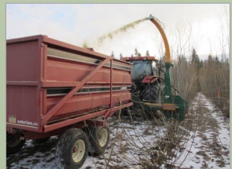
Figure 5. Willow harvest with modified sugar cane harvester
